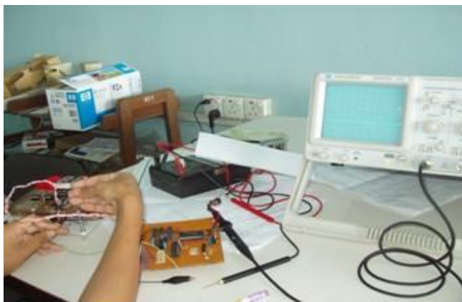
Fig. 15. Testing the received voltage level at the display unit.
